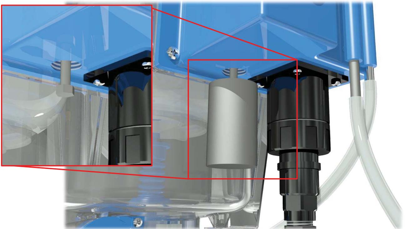
**Figure 140 – Location of the cap on the load cell calibration hook**
