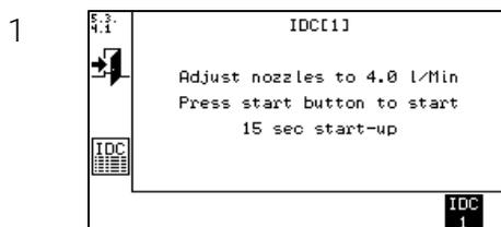
The flowmeter is set to suck through the large and the small nozzle at the same time. The flow meter will now suck 4 l/min. Press start and the IDC 2b or 3b will suck up testing liquid and will stop automatically after 15 seconds. (This is done to change the amount of testing liquid in the IDC 2b or 3b and change the hoses to a high flow).
