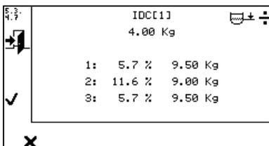
Occasional 3 or more calibrations must be conducted before the ✓ appears in the top right corner. Tests must be conducted until the ✓ appears else the measuring beaker have to be replaced.
