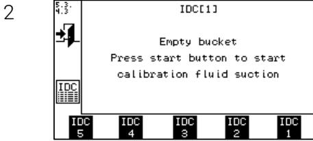
Empty the milk bucket on the floor and ensure that there is enough testing liquid in the bucket standing in the cow's place.
