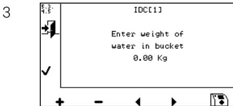
Weight out the amount of testing liquid (kg) in the milk bucket and enter the weight into the UniMilco. IDC 2b or 3b number is shown on top of the UniMilco Screen. After successful entry, the display image changes to the one in item 4.
