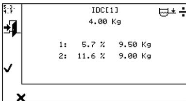
The bottom screen image appears if this part of the calibrations is inaccurate and must be repeated or enough measurements have not been made. As displayed there is no ✓ above the center button. Furthermore, there is a ÷ on top of the screen. It is only possible to leave the menu, which brings the IDC 2b or 3b back to step 1 item 2.
