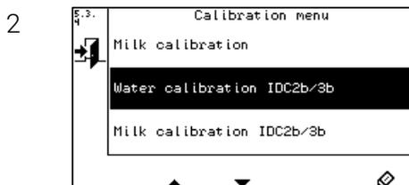
Chose 5.3.4 Water calibration IDC 2b or 3b and press in right bottom corner.
