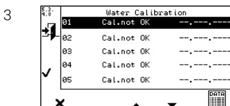
Chose up to 5 x IDC 2b or 3b for water calibration test
