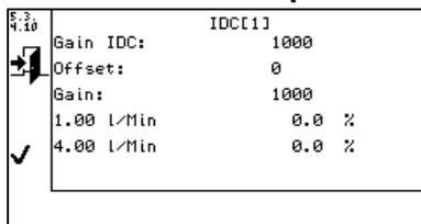
Gain IDC, Offset, Gains, 1,00 l/min and 4,00 l/min values can be seen for each IDC 2b or 3b in menu 5.3.4.10
