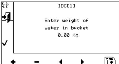
Weight out the amount of testing liquid (kg) in the milk bucket and enter the weight into the UniMilco. After successful entry, the display image changes to the one in item 4.
