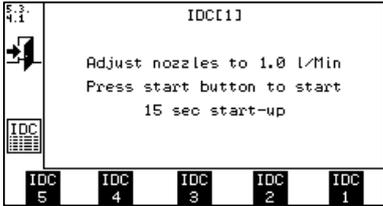
Set flowmeter to only suck through the small nozzle (flow meter will now suck 1 l/min). Press start, and the IDC 2b or 3b will suck up testing liquid for 15 seconds. The IDC 2b or 3b will stop automatically.
