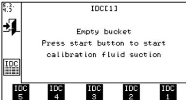
Empty the milk bucket on the floor and ensure that there is enough testing liquid in the bucket standing in the cow's place. Press the start button and the IDC 2b or 3b will start sucking up testing liquid from the bucket. The IDC 2b or 3b stops automatically, when 6 kg has been sucked through IDC 2b or 3b and screen image on UniMilco changes to the one displayed in item 3.
