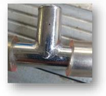
**Hoses and connectors** to set-up the test system – the milking bucket should have an inlet port of 20mm or more. Hence, the internal diameter of piping connecting between milk meter and bucket must be at least 20mm.
