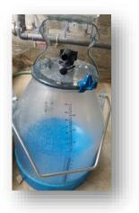
**Suction pipe** with an inlet hole of 3.5mm, which allows a  $4 \pm 1$  LPM (Liter per Minute) flow of water. The entire set should be tested and verified for the defined flow rate (see testing the
