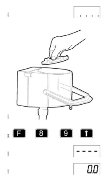
Check with a calibration weight that the milk meter displays the correct value.
