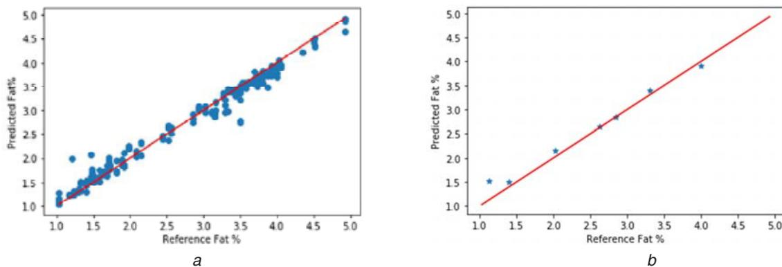
Figure 3. (a) Fat Calibration model with  $R^2$  of 0.984 and RMSE of 0.158. (b) Fat Validation results with  $R^2=0.991$ , RMSE = 0.167, Bias=0.096 and SEP=0.147
