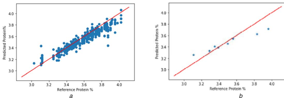
Figure 4. (a) Protein calibration model with  $R^2$  of 0.891 and RMSE of 0.078. (b) Protein validation results with  $R^2 = 0.979$ , RMSE = 0.127, Bias = -0.033 and SEP=0.131
