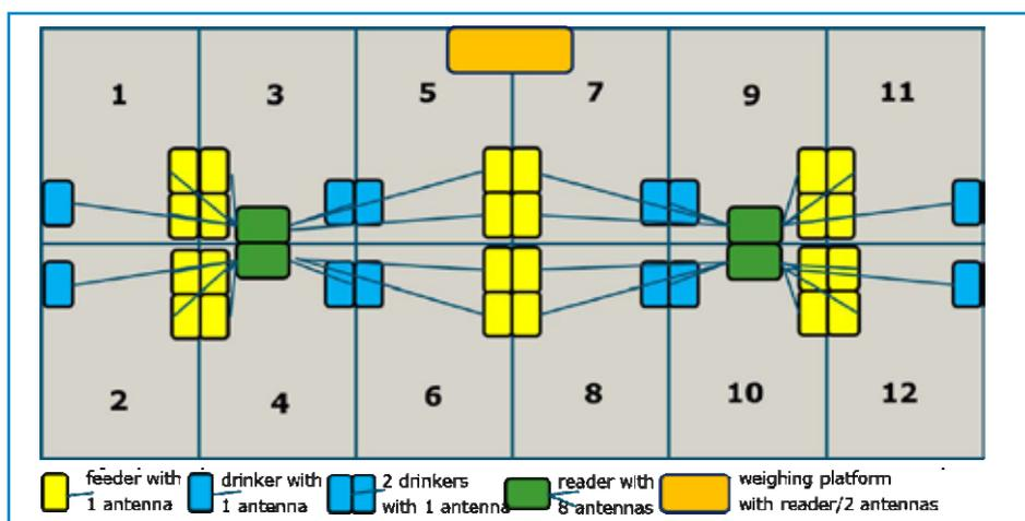
Figure 1. Layout of the barn with 12 pens each with one drinker and two feeders; 4 readers, each with 8 antennas; one weighing platform (with reader) connecting pens 5 and 7.
