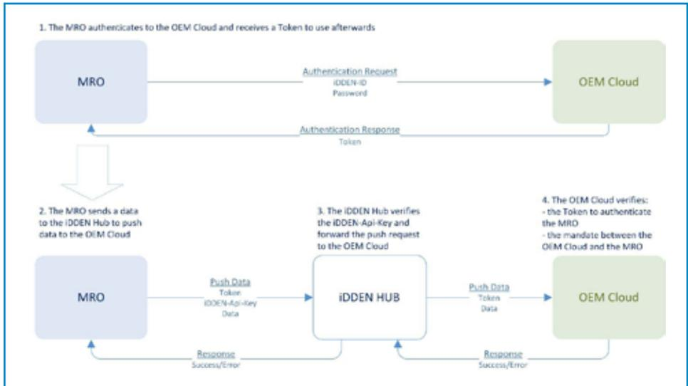
Figure 4. Send data from MRO to OEM Cloud.
