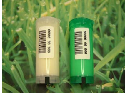
Vials colour coded – clear for quality testing, Green for composition testing. Tanker composite sample is pink.
