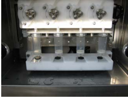
Fonterra 4 head automatic sampler. Other company's range from manual dip systems to semi automated systems.
