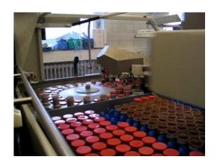
The ILAS robot will identify vials for special analysis, and after the CombiFoss (fat, protein, and cell count ) the racks are moved to the Pic and Place Robot
