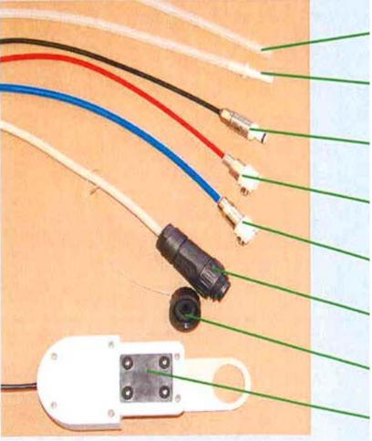
Tube for return air 100 cm Tube for milksample 150 cm Tube for moving glass wheel Tube for moving valve up and down
