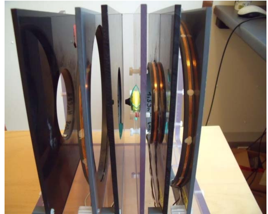
Helmholtz coil for ISO measurements of electronic ID devices
