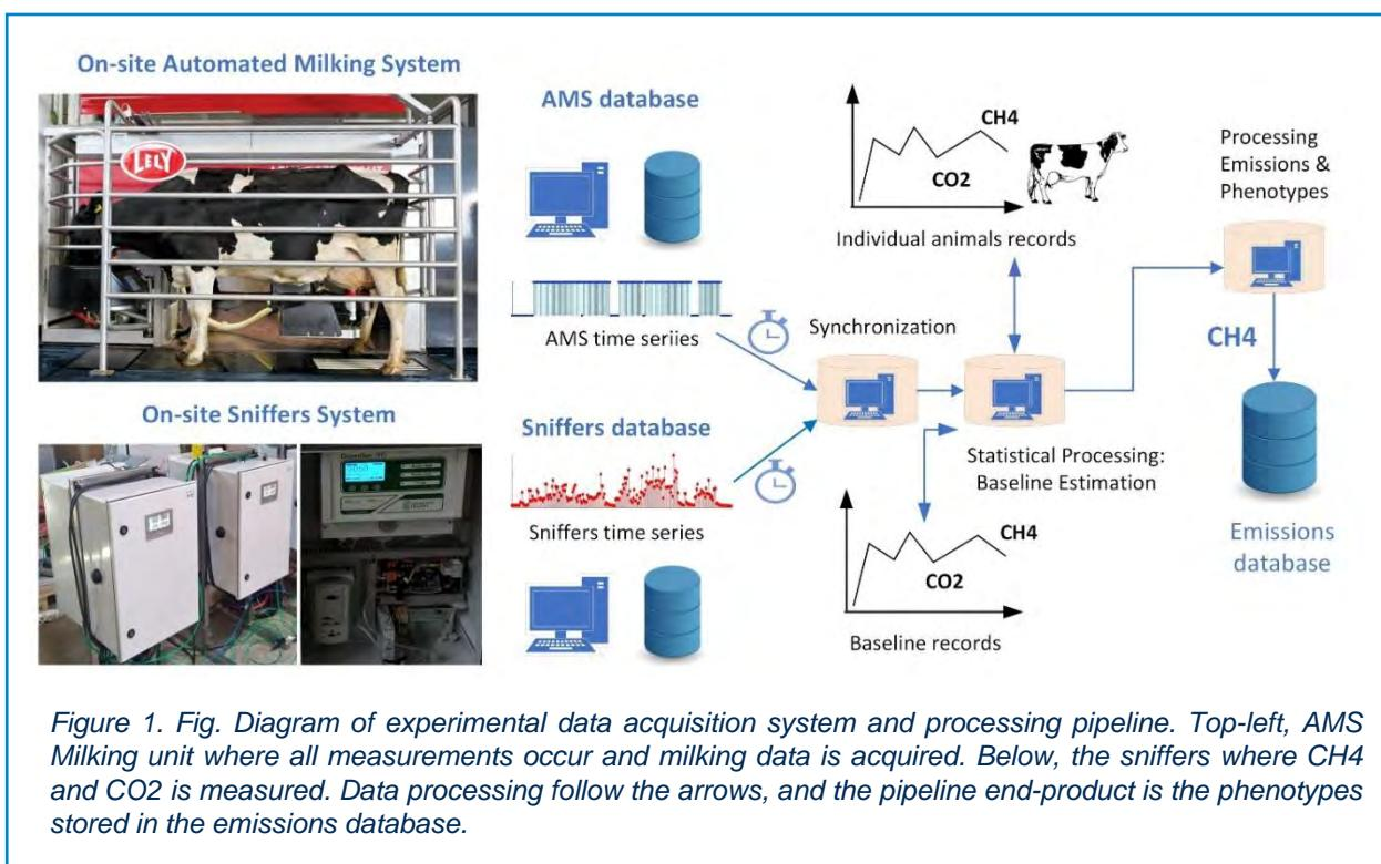
*Figure 1. Fig. Diagram of experimental data acquisition system and processing pipeline. Top-left, AMS Milking unit where all measurements occur and milking data is acquired. Below, the sniffers where CH<sub>4</sub> and CO<sub>2</sub> is measured. Data processing follow the arrows, and the pipeline end-product is the phenotypes stored in the emissions database.*
