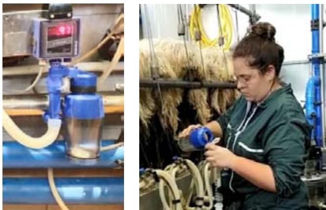
Figure 3. Sampling in electronic meter milking machine.
