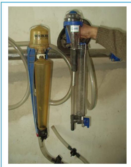
Figure 2. Main brands of mechanical milk meters used in Uruguay, Waikato® (left), Tru Test® (right).
