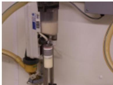
The meter then fills the vial, empties the flask and is ready for the next cow. This process takes about 10 seconds.
