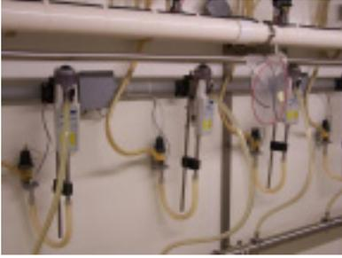
When this herd expanded the parlor the vacuum shutoffs were going to be mounted right on the milking line. When we told the dairyman we needed vacuum 100% of time to agitate the samples and would need to go back to using the pull out meters the dairyman made the dealer mount the vacuum shutoffs on the wall.
