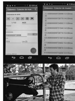
Photo 1. The first main display of smartphone app, second info codification display. Below RFID capture process in milking room parlor.
