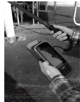
Photo 2. Device-type smartphone with a cane to capture the data of the ears identification tags of each cattle through RFID and milk samples, with a barcode on each vial, which is used by the milk production controller in the dairy barn.
