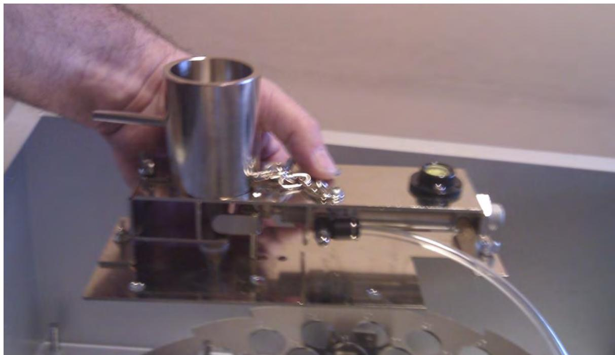
Use the syringe to inject hot water with a little acid in the silicone hoses and in the stainless steel tank.
