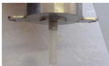
Please remove the silicone hose and replace it on the tank filler (without silicone grease)
