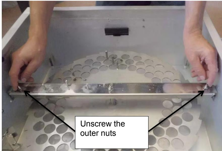
To remove the crown, it is necessary to tilt it to one side.
