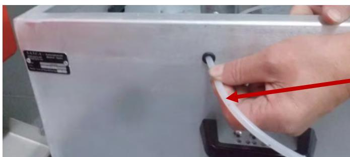
Place the milk hose in the hole that is protected by a rubber ring
