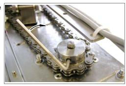
• Re-assemble the sampling device.
