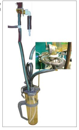
• Remove hose from the right-hand connector on the sampler
