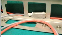
• Alternatively, the plug may be fastened to the positioning device with a cable tie.
