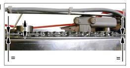
• Tighten the threaded pin on the sprocket (drive) with a spanner.
