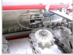
Change the position of the limit switch so that the filling nozzle is exactly on the marking for the first filling position.
