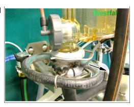
• Fasten sample tank to the sampler with holder and knob.
