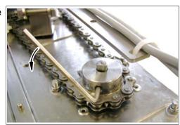
• Place a spanner on the square of the chain tensioner and loosen the chain.
