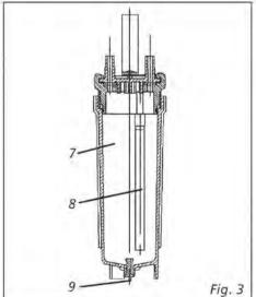
By rotating the sample reservoir four different functions can be set. The relevant positions are marked on the cover plate.
