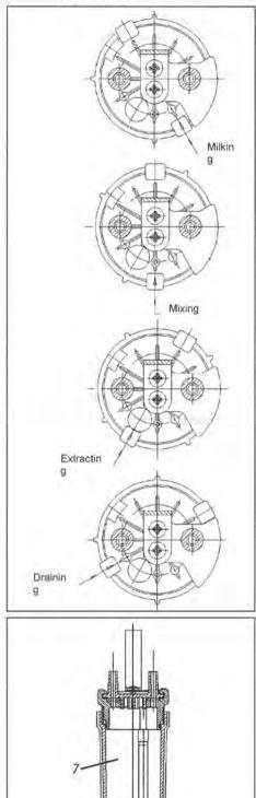
By rotating the sample reservoir four different functions can be set. The relevant positions are marked on the cover plate.
