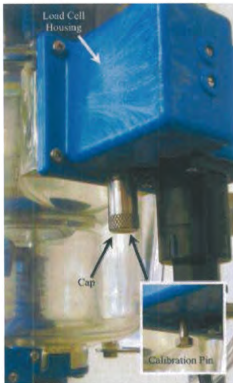
Figure 37 Cap on load cell housing.
