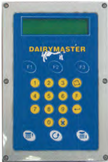
Figure 5 Weighall milk meter control panel.
